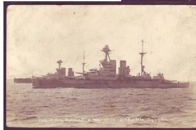
Queen Elizabeth class Battleships were 27,500 tons and had a speed of 25 knots, armed with eight 15inch and sixteen 6inch guns and were the most powerful ships at Jutland. Completed 1915.
