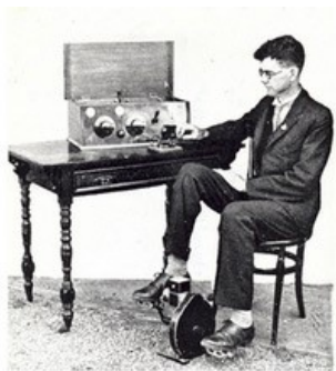
Alfred Traeger's Pedal Powered Radio in 1929. Photo courtesy of the Royal Flying Doctor Service.
